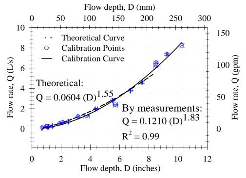
Figure 9 Parshall flume calibration curve
