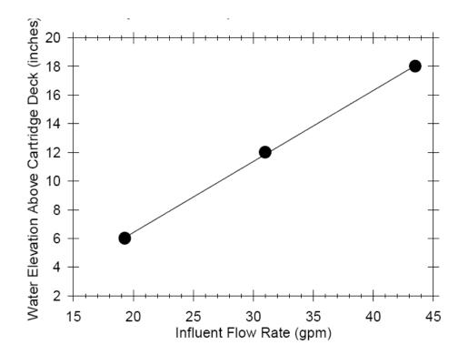
Figure B1: Hydraulic response of a clean 54-inch long Jellyfish filtration cartridge with a 35 mm lid orifice, used as the draindown cartridge in the JF4-2-1.
