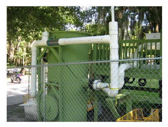
Figure 6 Photo of field test set-up for the Jellyfish<sup>®</sup> Filter JF4-2-1. Below-deck inlet pipe enters the right side of the vessel and outlet pipe (invert at deck level) exits the left side of the vessel. External bypass piping has invert of horizontal section 18 inches above deck level.
