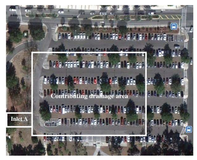
Depending on the storm event intensity and wind direction the drainage area can vary from 5,400 to 8,600 ft<sup>2</sup> (0.12 to 0.20 acres) of pavement. The catchment drains to inlet A as shown in Figure 4(b) and 4(a). Runoff captured by inlet A is the source of influent to the downstream Jellyfish Filter.
