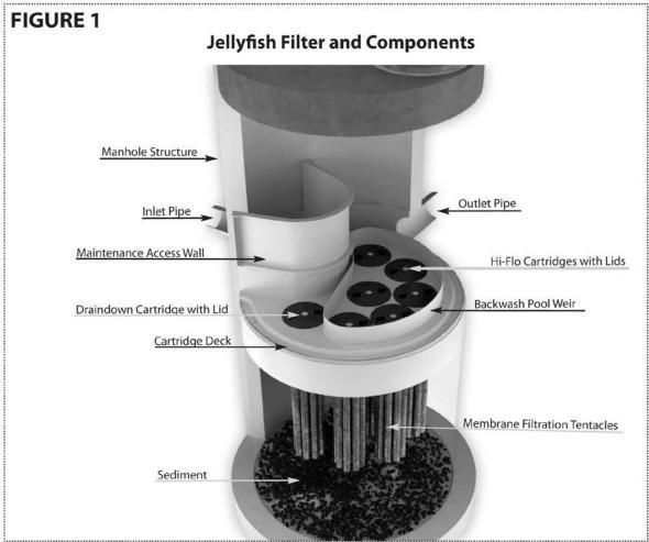
Figure 1 Jellyfish<sup>®</sup> Filter and Components
