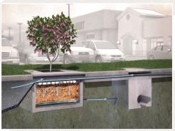
Filterra System showing curb-inlet opening.
