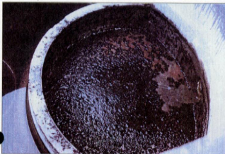
PLATE 6: View of inlet following drain down after inorganic sediment retention test.
