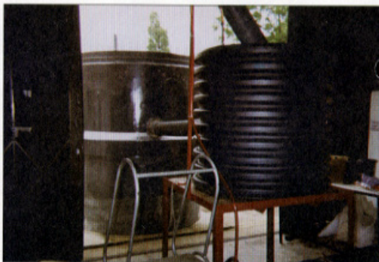
PLATE 1: General view inside the Hydraulics Laboratory showing the drum of test oil (right); the inlet/mixing tank on the red frame with the oil feed pipe and grey water supply pipe (centre); and the X-Ceptor unit in the doorway.
