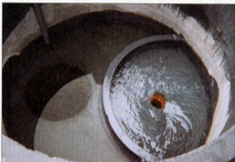
PLATE 3: A view inside the bypass chamber during tests with organic sediment additions, revealing the bypass overflow weir, the small diameter inlet and large diameter outlet pipes from the treatment chamber.
