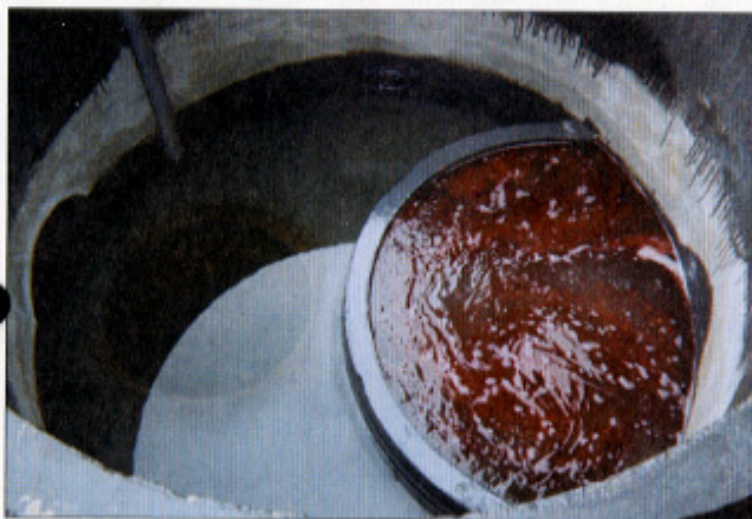
PLATE 5: View of inlet during tests with the addition of organic sediment (peat) showing vortex above inlet pipe to treatment chamber.
