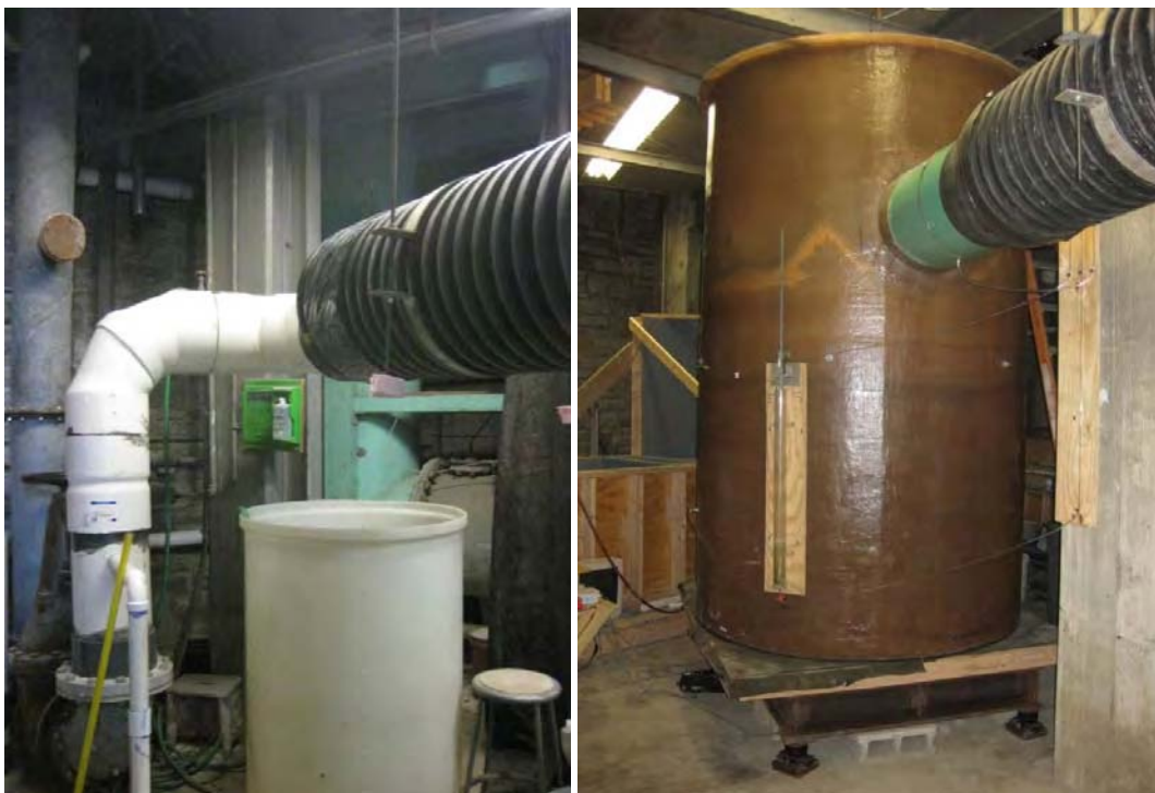
Figure A-11: Stormceptor water feed piping
