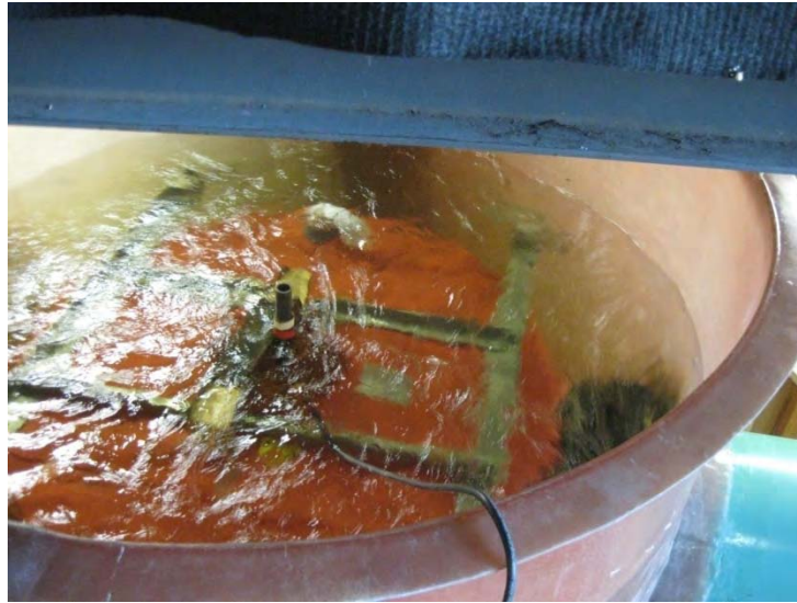
Figure A-19: Water flowing through Downstream Defender during the laboratory tests
