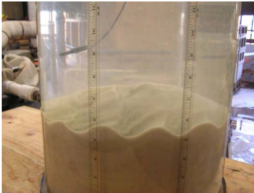
Figure 4-2: Bedforms in swirl flow device scale model
