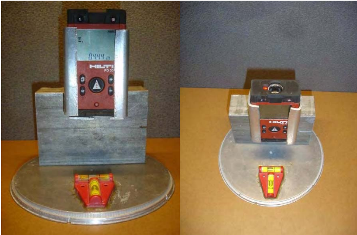
Figure C-2: Laser range finder with bracket
