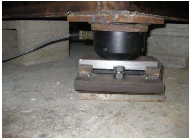
Figure C-3: Load cell installed under device
