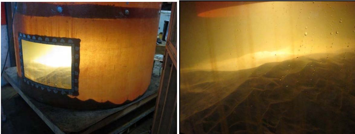
Figure A-20: Bedforms in the sump of Downstream Defender at high flow conditions
