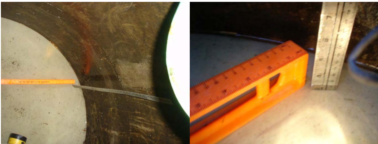
Figure C-1: Sediment depth measurement using the metal ruler stick
