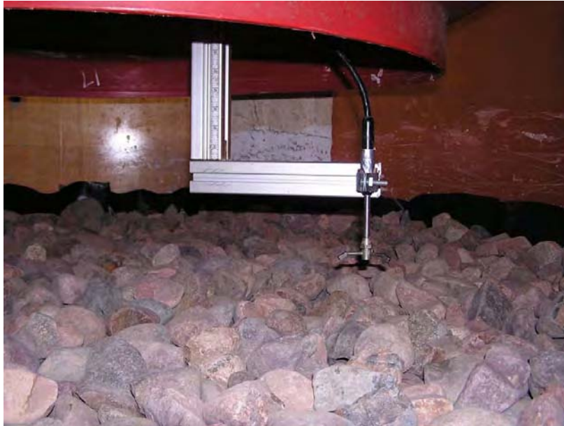
Figure 5-6: ADV positioned above the river rock bed
