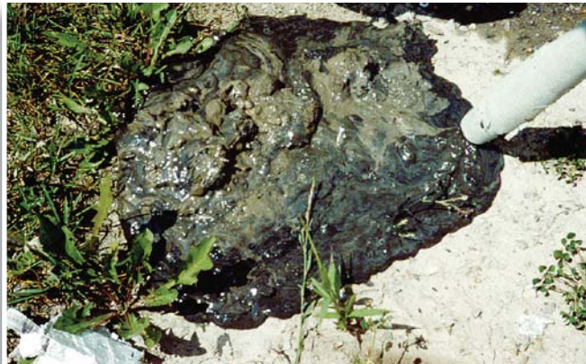
The pollutant-laden sediment captured by a stormwater treatment device is often tar-like and toxic.
