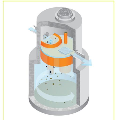
When the snow pile melts in the spring, the runoff flows down a specially-constructed asphalt pad to a series of catch basins and the Stormceptor. The Stormceptor slows the water and allows free oils to rise while sediment, with associated heavy metals and nutrients, settle and are held safely in the treatment chamber. The water then flows to a treatment pond for further treatment, and into a closed storm sewer system before discharging as clean water into a tributary of the Rouge River.
