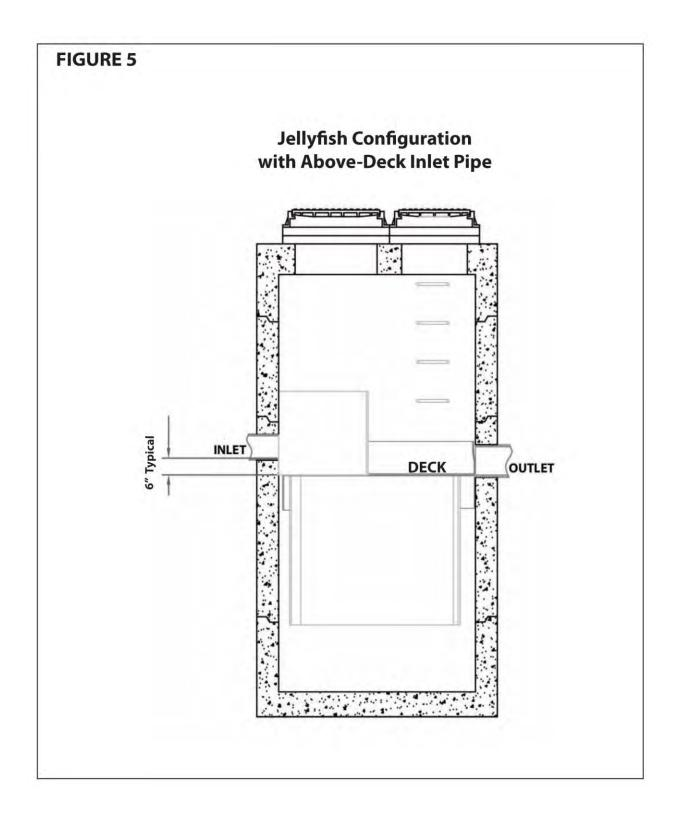
For the standard above-deck inlet pipe configuration, the invert elevation of the inlet pipe is typically set 6 inches (150 mm) higher than the invert elevation of the outlet pipe. This generally ensures that the inlet pipe will drain completely at the conclusion of each rainfall/runoff event, while providing sufficient volume within the maintenance access wall zone for surface accumulation of floatables below the inlet pipe. The elevation of the inlet pipe can be varied as required.
