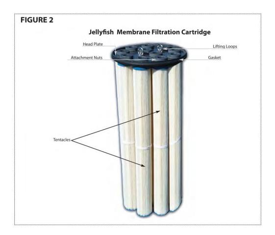
The filtration tentacle membranes provide an extraordinarily large amount of surface area, resulting in superior flow capacity and suspended sediment removal capacity. A typical Jellyfish cartridge with eleven 54-inch (1372 mm) long filtration tentacles has 381 ft2 (35.4 m2) of membrane surface area. Hydraulic testing on a clean 54inch (1372 mm) filter cartridge has demonstrated a flow rate of 180 gpm (11.3 L/s) at 18 inches (457 mm) of driving head.
