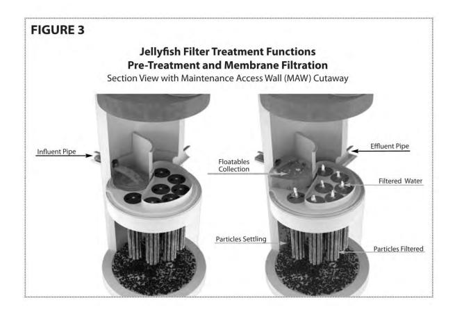
**Pre-treatment** removes coarse sediment (generally > 50 microns), particulate-bound pollutants attached to coarse sediment (nutrients, toxic metals, hydrocarbons), free oil and floatable trash and debris. These pollutants are removed by gravity separation. Large, heavy particles fall to the sump (sedimentation) and low density pollutants rise to the surface (floatation) within the pre-treatment channel.
